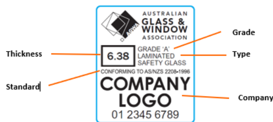
Figure 1 Example of safety label applied to Post Cut Laminated Glass
